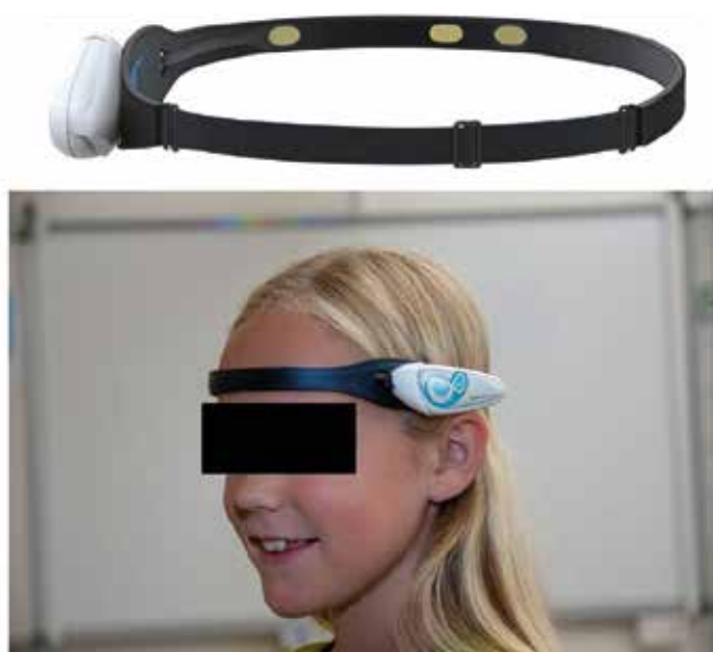
Wearable electroencephalographic (EEG) device for detection of absence seizures using artificial intelligence.
